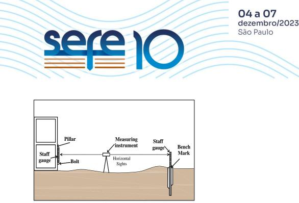
Figure 11 – Illustration of the geometric leveling method
