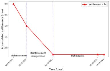
Figure 12 – Settlement suffered by the P4 pillar
