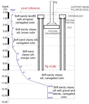
Figure 10 - AA Section - Geotechnical Profile
